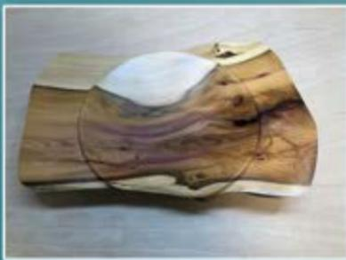
The large split log at the top of this article has now had a few rough edges and loose bark taken off and is mounted on my lathe ready for attention. Slow speed required!
