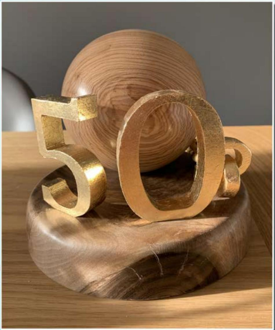
The ball was roughly turned to an approximate sphere and then refined using a simple jig that I made up as illustrated in the following images. The first image shows how the wood is held between centres to refine the shape of the sphere,
